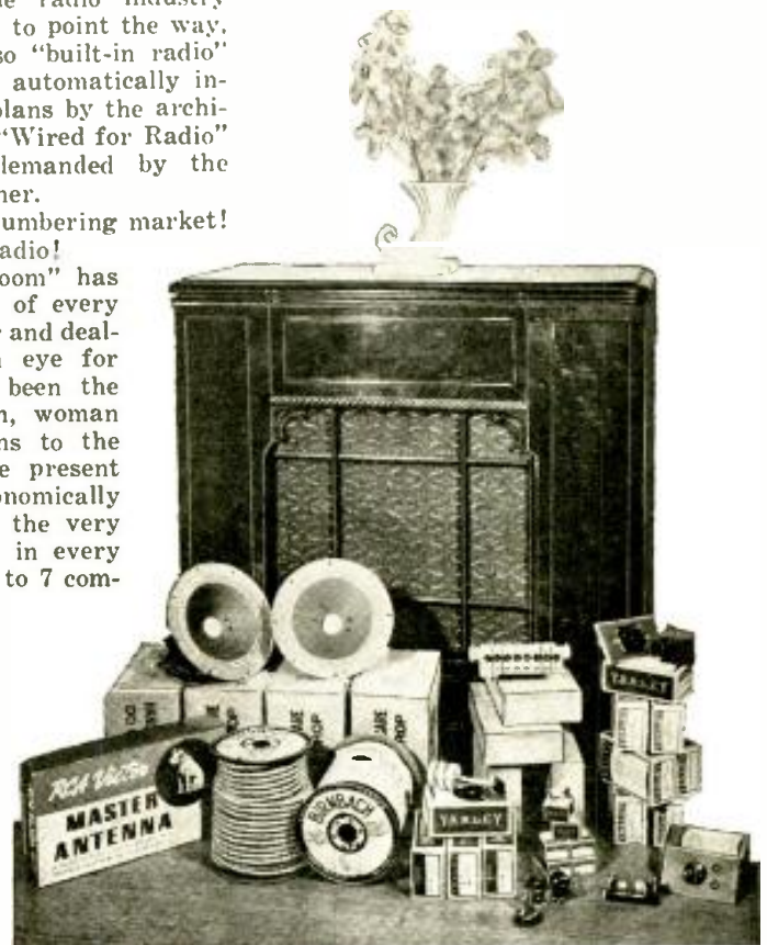
These are the major components of the built-in radio system. In the background is the beautiful RCA-Victor high-fidelity victrola-radio combination model U-130. In front of it are 6 (7 will be used) RCA P.-M. dynamic speakers; 6 Mallory-Yaxley pushbutton switches, multi-contact outlets, pilot light sockets, and combination power and combined "Ant.-Gnd." outlet; Birnbach 7-wire shielded cable; RCA-Victor master antenna; and relay for turning the set on and off, remotely.
